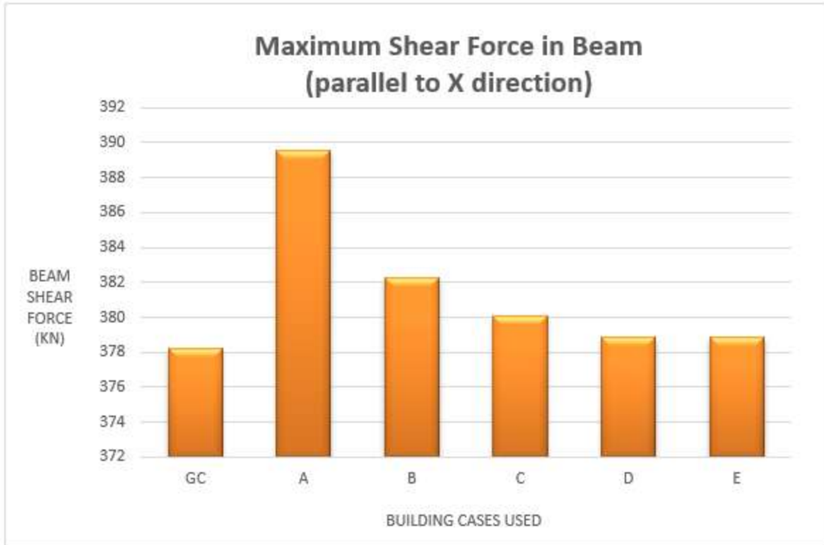
Fig. 10: Maximum Shear Forces in beams parallel to X direction for all Building cases
